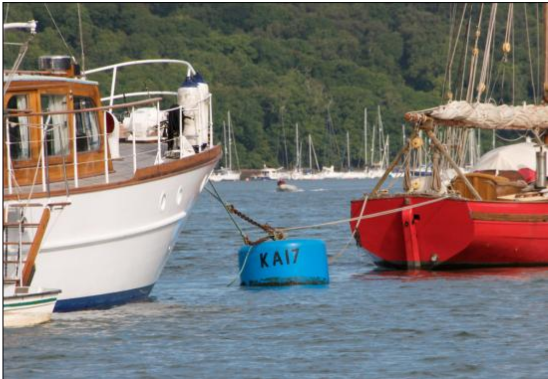
Vessels moored to a typical Dart Harbour mooring buoy
