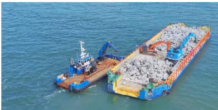
Aarsleff 120 barge with Hound Dog Tugboat carrying 1-3T rock armour.
